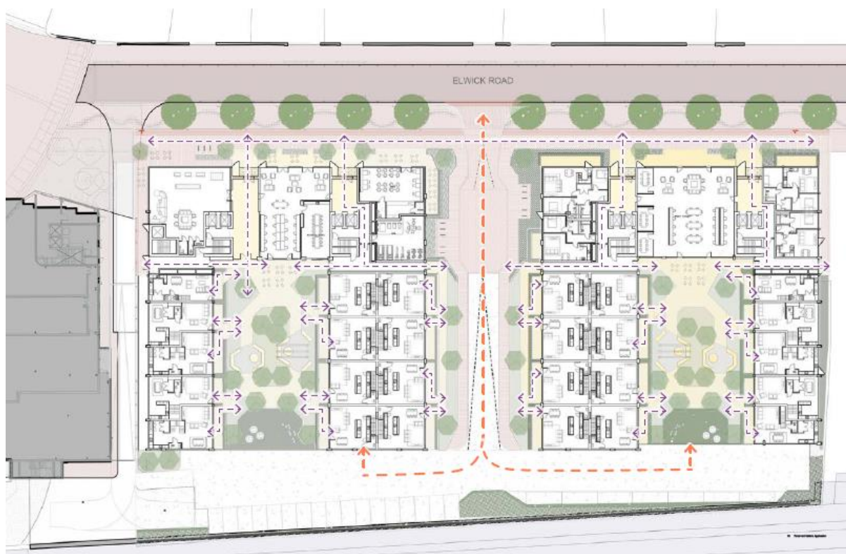
Figure 2: Inclusive Access (Upper ground floor)
